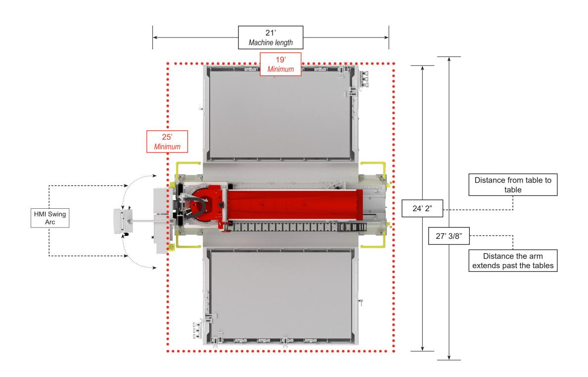
NOTE: Red border indicates the minimum continuous 6" slab required.
